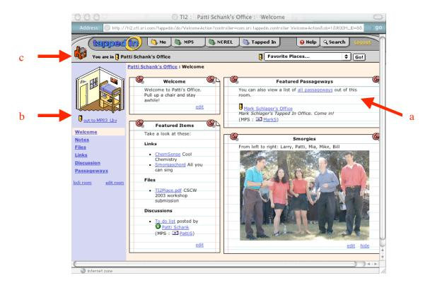
**Figure 5**. Redesigned TI2 Office with (a) separated Passageways note, (b) new "out" link to the new lobby of the 3<sup>rd</sup> floor on which it resides, and (c) icon corresponding to current building (previously, this icon was tied to the customizable room look and feel). (Chat disabled to highlight changes.)
